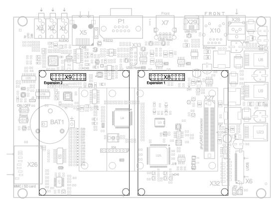
Figure 10: Expansion connector X8A, X9A
