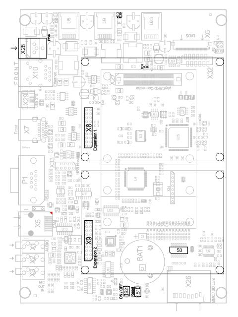
Figure 8: phyBASE Overview of applicable Connectors, LEDs and Buttons
