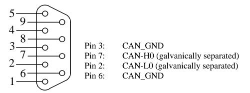
Figure 4: Pin Assignment of the DB-9 Plug X1
