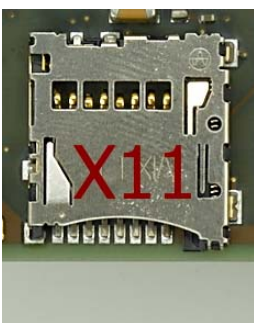
Figure 11: SD / MM Card interface at connector X11
