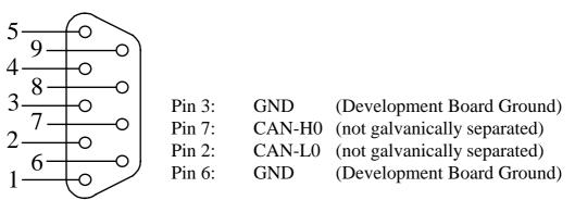
Figure 20: Pin Assignment of the DB-9 Plug P2A (CAN Transceiver on phyCORE-167HS/E, Front View)
