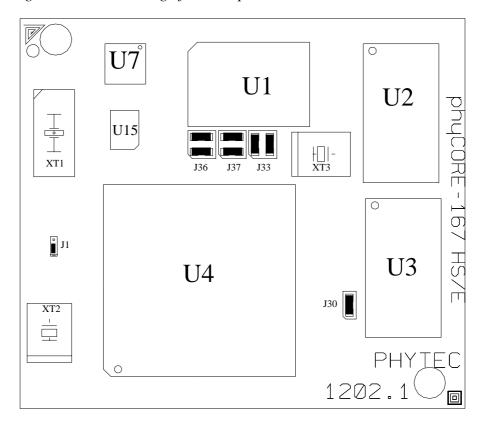
Figure 6: Location of the Jumpers (Controller Side)
