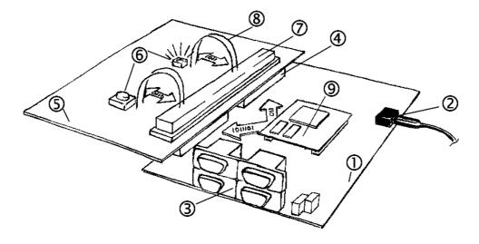
Figure 10: Modular Development and Expansion Board Concept with the phyCORE-167HS/E
