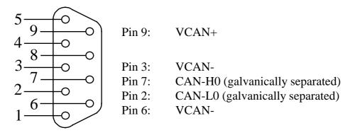
Figure 22: Pin Assignment of the DB-9 Plug P2A (CAN Transceiver on Development Board with Galvanic Separation)
