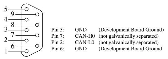
Figure 21: Pin Assignment of the DB-9 Plug P2A (CAN Transceiver on Development Board)
