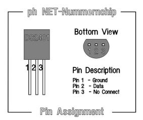
Figure 29: Pin Assignment of the DS2401 Silicon Serial Number
