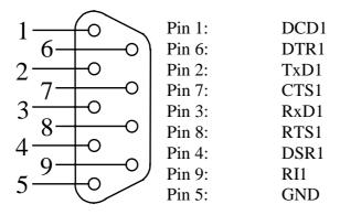
Figure 18: Pin Assignment of the DB-9 Socket P1B as Second RS-232 (UART Populated, Front View)
