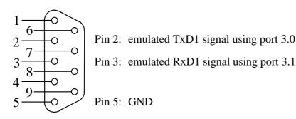
Figure 19: Pin Assignment of the DB-9 Socket P1B as Emulated RS-232 (Front View)
