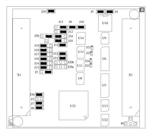
Figure 7: Location of the Jumpers (Connector Side)
