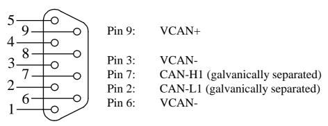
Figure 25: Pin Assignment of the DB-9 Plug P2B (CAN Transceiver on Development Board with Galvanic Separation, only with C167CS)
