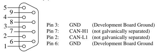
Figure 24: Pin Assignment of the DB-9 Plug P2B (CAN Transceiver on Development Board, only with C167CS)
