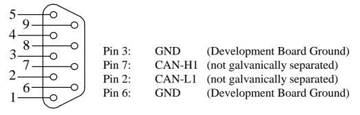
Figure 23: Pin Assignment of the DB-9 Plug P2B (CAN Transceiver on phyCORE-167HS/E, only with C167CS)
