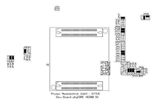
Figure 14: Default Jumper Settings of the phyCORE Development Board HD200 with phyCORE-167HS/E
