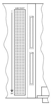
Figure 27: Pin Assignment Scheme of the Patch Field
