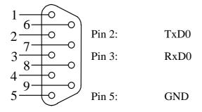
Figure 16: Pin Assignment of the DB-9 Socket P1A as First RS-232 (Front View)
