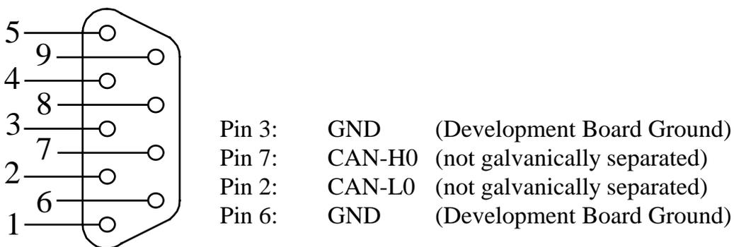
Figure 20: Pin Assignment of the DB-9 Plug P2A (CAN Transceiver on phyCORE-167HS/E, Front View)
