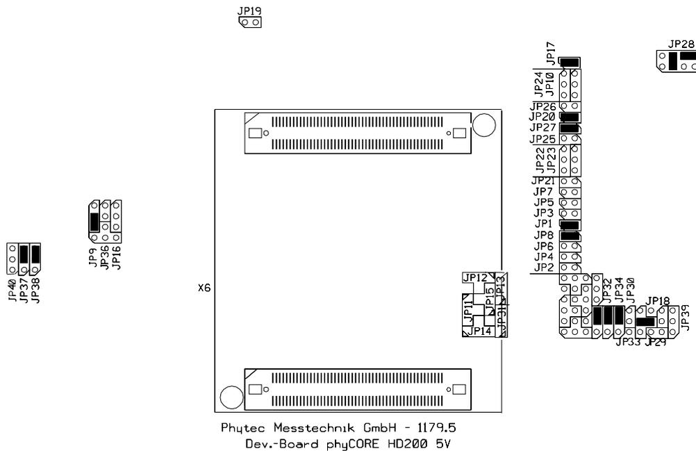
Figure 14: Default Jumper Settings of the phyCORE Development Board HD200 with phyCORE-167HS/E
