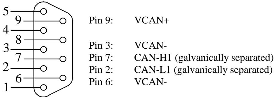
Figure 25: Pin Assignment of the DB-9 Plug P2B (CAN Transceiver on Development Board with Galvanic Separation, only with C167CS)
