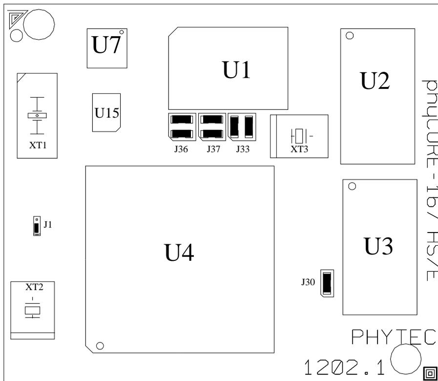
*Figure 6: Location of the Jumpers (Controller Side)*
