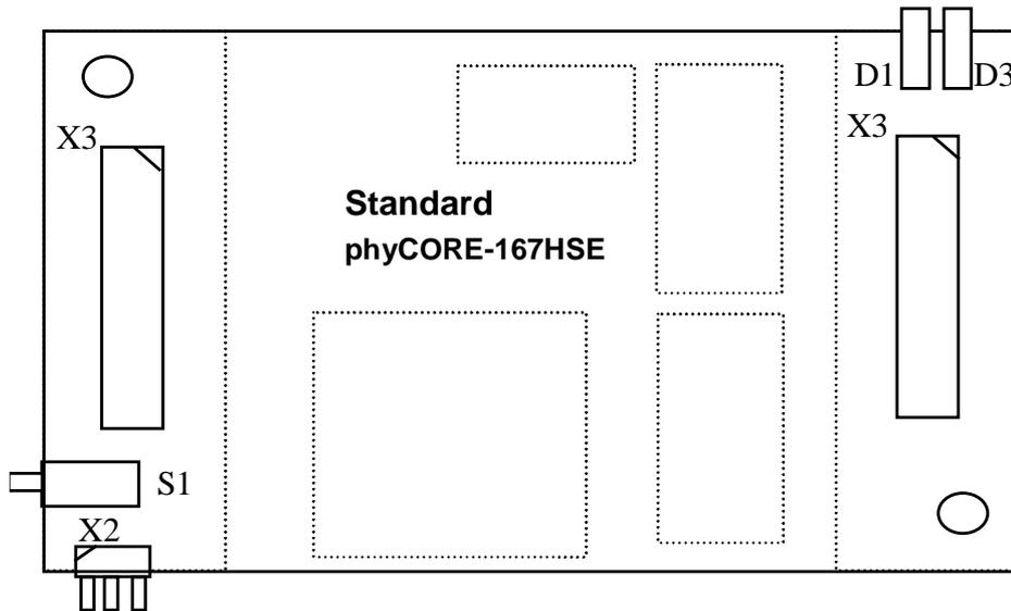
Figure 30: Positions of the Additional Components on the debugCORE-167HSE
