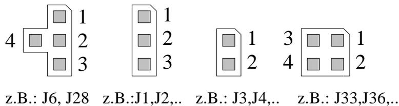
*Figure 5: Numbering of the Jumper Pads*
