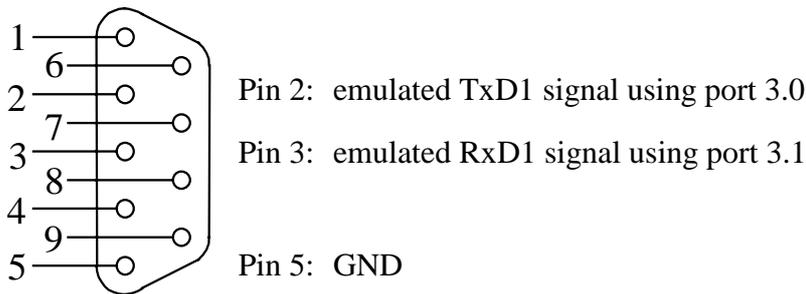
Figure 19: Pin Assignment of the DB-9 Socket P1B as Emulated RS-232 (Front View)
