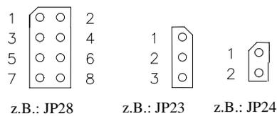
Figure 12: Numbering of Jumper Pads
