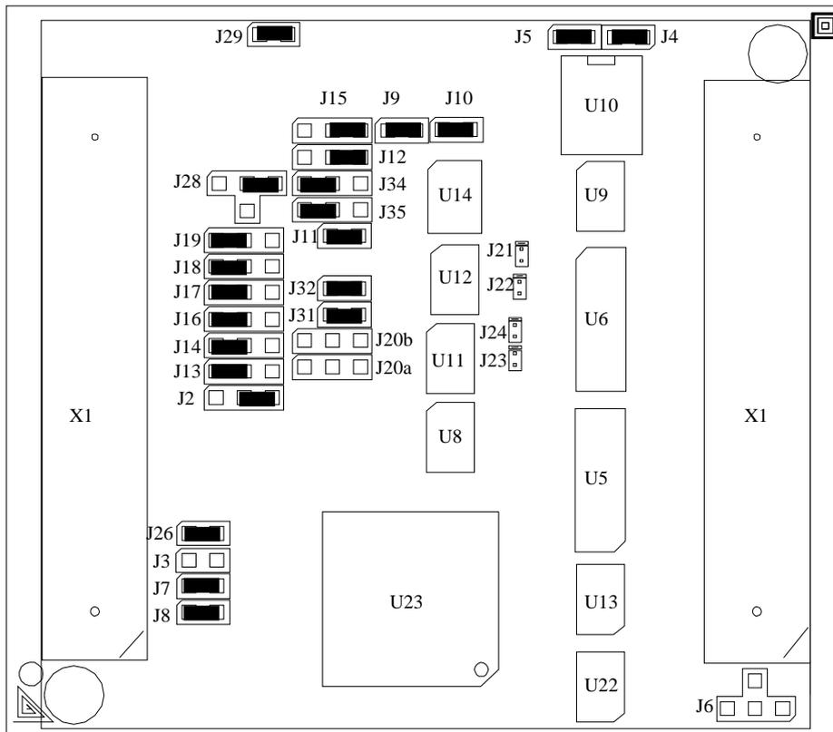
Figure 7: Location of the Jumpers (Connector Side)
