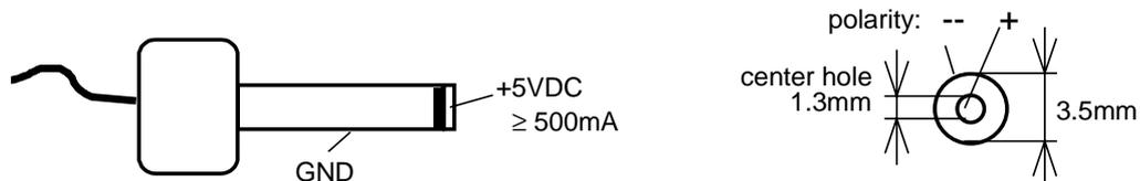
Figure 15: Connecting the Supply Voltage at X1
