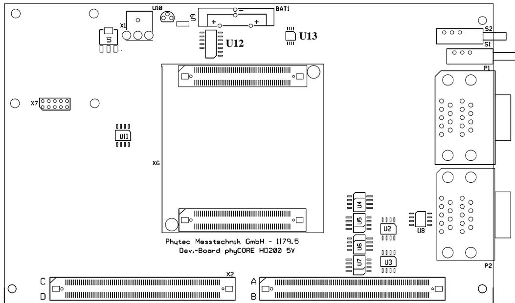
Figure 17: Location of Components at U12 and U13 for Power Supply to External Subassemblies
