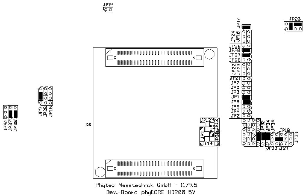
Figure 15: Default Jumper Settings of the phyCORE Development Board HD200 V3 with phyCORE-XE167
