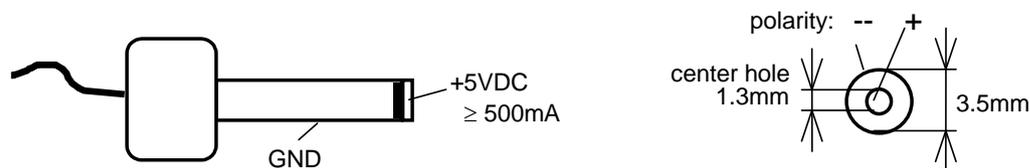
Figure 16: Connecting the Supply Voltage at X1
