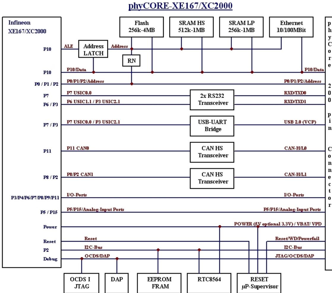
Figure 1: Block Diagram phyCORE-XE167
