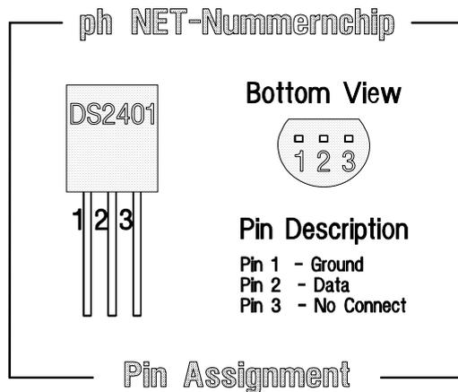
Figure 34: Pin Assignment of the DS2401 Silicon Serial Number
