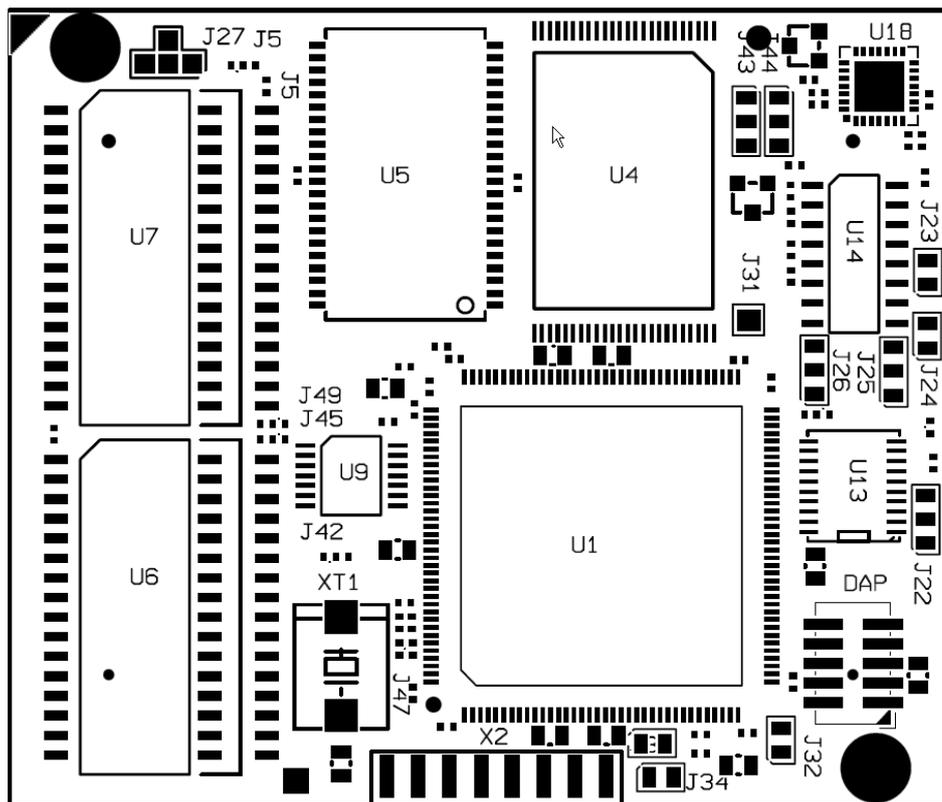
*Figure 6: Location of the Jumpers (Controller Side Top View)*
