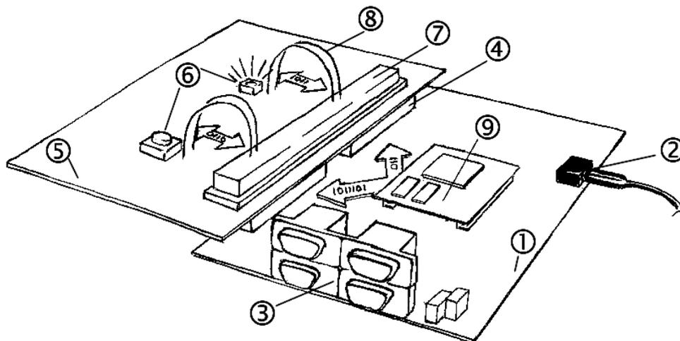
Figure 11: Modular Development and Expansion Board Concept with the phyCORE-XE167
