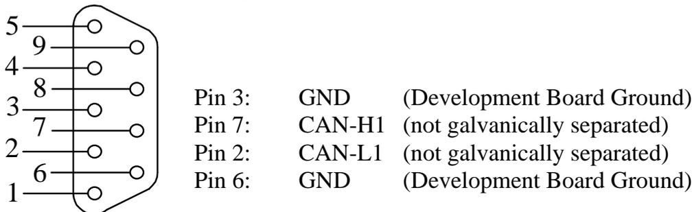
Figure 24: Pin Assignment of the DB-9 Plug P2B (CAN Transceiver on phyCORE-XE167)
