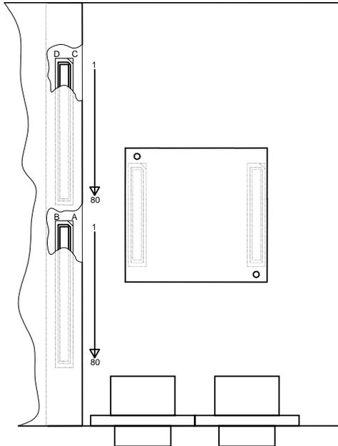
Figure 26: Pin Assignment Scheme of the Expansion Bus
