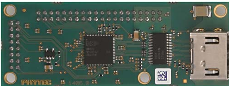
Figure 10: View of the HDMI Adapter (PEB-AV-01)
