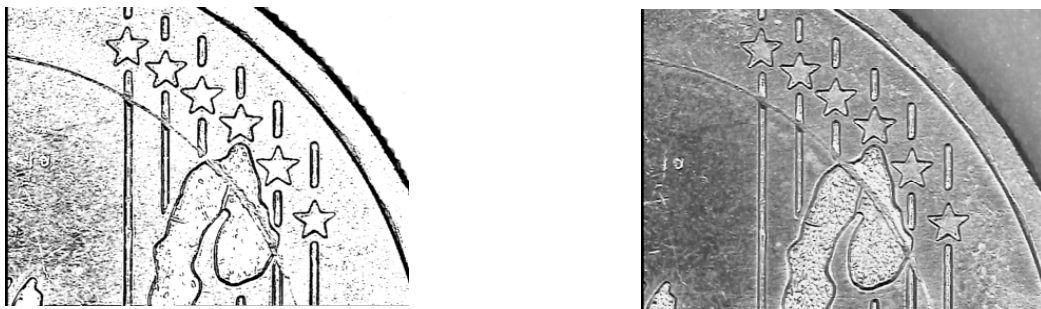
Figure 6: Coin with Focussed Lighting (Photograph to the Left, Quality is Worse) and Diffused Lighting (Photograph to the Right, Quality is Better)
