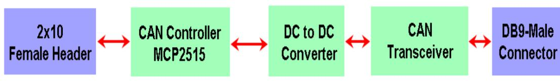
Figure 2: Block Diagram PEB-A-001
